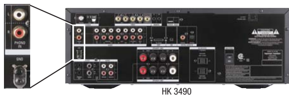
Figure 14 – Phono Inputs and Ground
