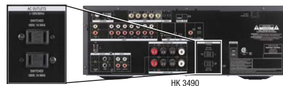
Figure 24 – AC Switched Accessory Outlets
